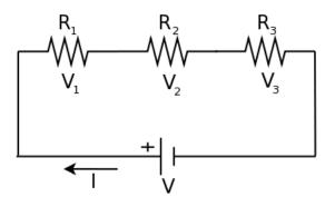
$V = V_{1} + V_{2} + V_{3} \text{ and current remains same}$ => But, V = I\*R, V<sub>1</sub> = I\*R<sub>1</sub>, V<sub>2</sub> = I\*R<sub>2</sub>, V<sub>3</sub> = I\*R<sub>3</sub> => I\*R = I\*R<sub>1</sub> + I\*R<sub>2</sub> + I\*R<sub>3</sub> => I\*R = I\*(R<sub>1</sub> + R<sub>2</sub> + R<sub>3</sub>)  $\Rightarrow R = R_{1} + R_{2} + R_{3}$
